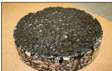
(c) Finished Scraped Core
