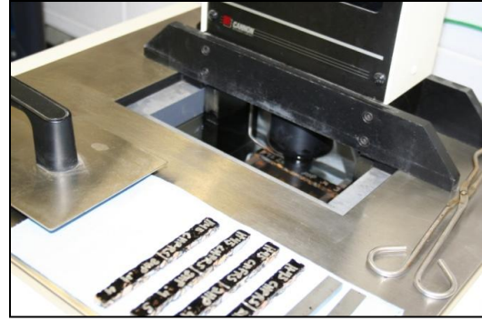
(b) Mixture Beam Testing
