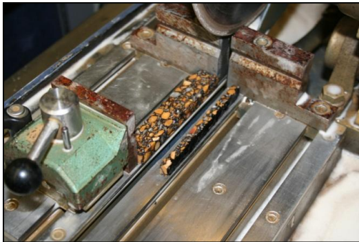
(e) Final Cut Producing BBR Mixture Beam
