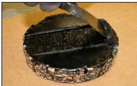
(a) Scraping Treated Core
