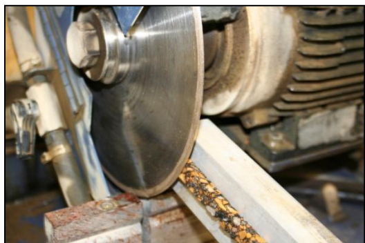
(e) Final Cut Producing BBR Mixture Beam
