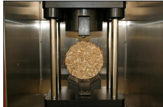
(b) Indirect Tensile Strength Testing
