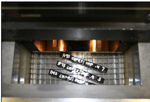
(e) Beams Conditioning in Methanol Bath
